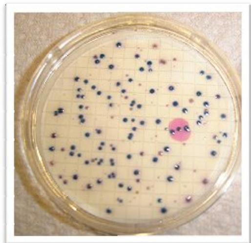
A sample of a test on streamwater approx two weeks after range cattle occupied upstream area. 10/100 ml dilution. Dark blue represents a fecal coliform count of approx 860 colonies per 100 ml
